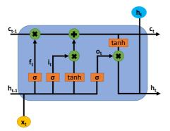
Figure. 2. The fundamental LSTM unit.
